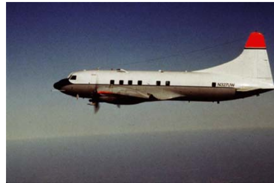
Figure 2. The Convair C-131A, 1950's airliner, CV-240, later converted to medical evacuation, "Samaritan." Like the B-23, it was sturdy and amenable to modification. Sadly, it was driven from the air by its thirst for high-octane leaded gasoline.
